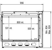
For the e-MatriX series, whilst stocks last, the fire casing may be 32mm lower than noted on the drawings in these brochures. After delivery, check the height of the fire casing to prevent misunderstandings. The very latest drawings of Faber fires are available on the website www.faberfires.com
